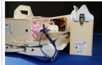
IGAR manipulator and full breast intervention platform mounted on the patient support structure with a biopsy tool attached.
